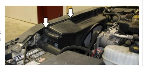
10. Unclip the transmission control module from the cover if required for access. Disconnect the top (RED) electrical connector.
