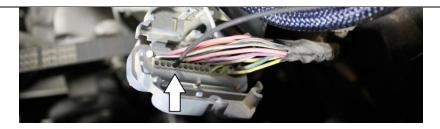
36. Clip the clamshell back together. Reinstall the clear retainer clip. Reattach to TCM.
