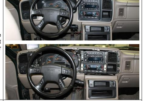
Remove the two 7mm screws from the bottom of the knee bolster and pull bolster outwards.
